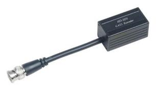
HD-SDI CAT5 Extender is a passive device which use in one pair to send HD-SDI signals up to 45m via a CAT6 cable at HD resolution in a point-to-point configuration. The HD-SDI passive CAT5 extender supports uncompressed transmission of up to 1.485G b/s. It is perfect to send HD CCTV over existing CAT5 cable Applications include HD-CCTV, broadcasting, HD camcorder, studio-to-studio, post production, live events, medical imaging displays, and medical imaging...etc.
